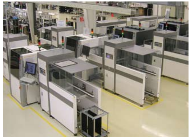
Four Viscom type S6056 DS2W systems in off-line operation
