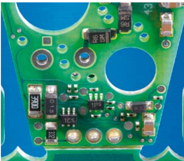
Lead-free ignition electronics with 0201 assemblies
